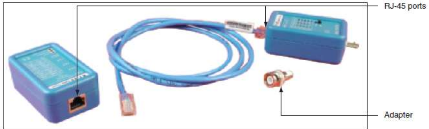
Figure 9-47 Use a cable tester pair to determine the type of cable and if the cable is good
