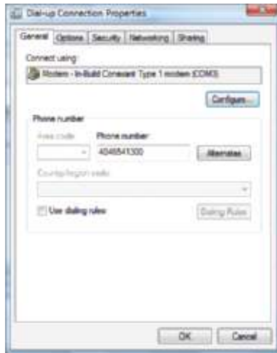
Figure 9-19 Configure an Internet connection using the Properties window of the connection icon Courtesy: Course Technology/Cengage Learning
