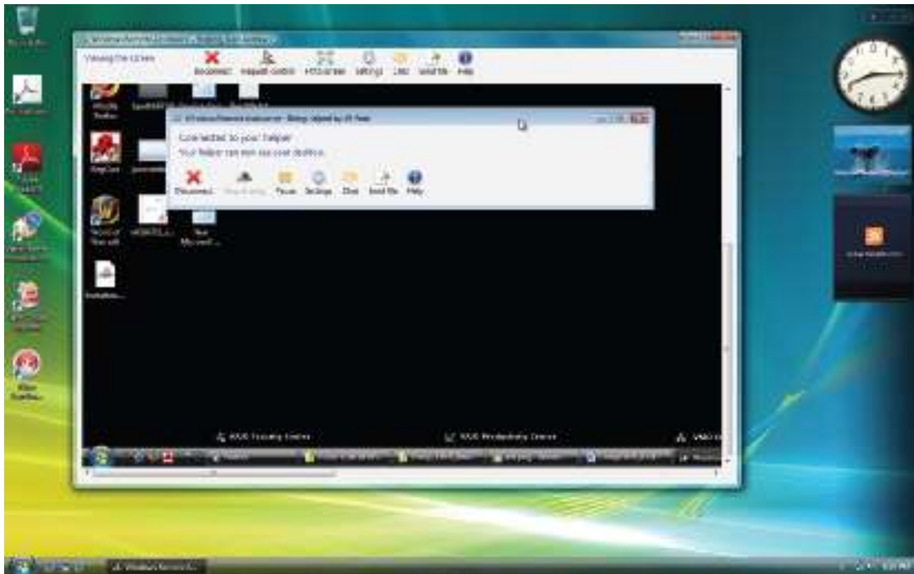
Figure 9-66 The user's desktop can be viewed by the support technician Courtesy: Course Technology/Cengage Learning
