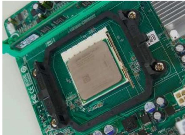
Figure 4-1 An AMD Athlon 64 X2 installed in socket AM2+ with cooler not yet installed Courtesy: Course Technology/Cengage Learning
