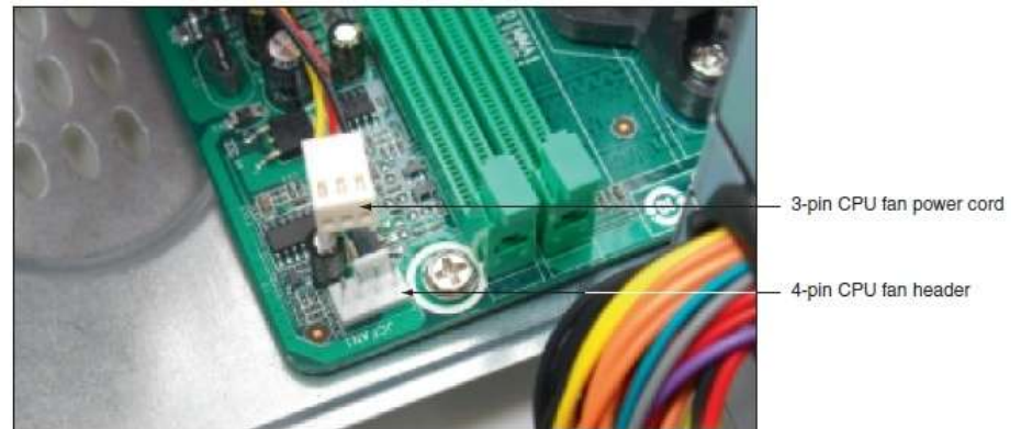
Figure 4-12 A cooler fan gets its power from a 4-pin PWM header on the motherboard Courtesy: Course Technology/Cengage Learning
