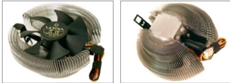
Figure 4-9 A cooler sits on top of a processor to help keep it cool Courtesy: Course Technology/Cengage Learning
